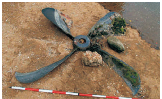
Figure 22. Whale chaser propellers discarded on the beach. The survey identified that different designs of propellers were present. These propellers are possibly a later design (ie. late 1920s) as they are made of an alloy and are a sleeker more light weight design. Other propellers are a more robust solid steel design and appear to be much heavier (Photo: NZHPT).
