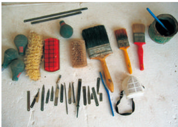
Tools used to remove the oil paint from wooden surfaces
