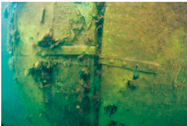
Figure 35. Intact rudder, starboard side showing pintle & gudgeon (Photo: SCHIP & Subsurface Ltd).
