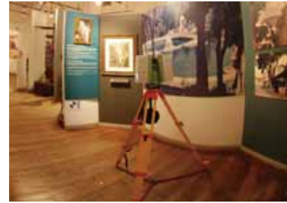
3D terrestrial laser scanner is placed inside the building to collect data in point cloud form through millions of laser pulses or distance measurements.
