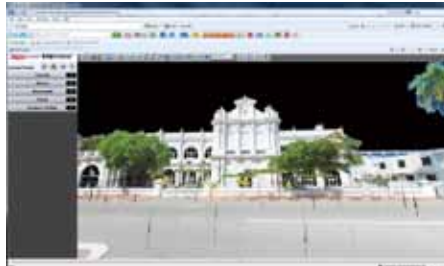
The front elevation of the building in true colour of point cloud
