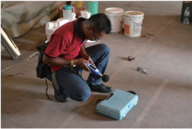
Several noise level experiments were carried out by experts at St. Mary's Cathedral in order to determine the noise level caused by the activities at the nearby Dataran Merdeka, and to gauge the effectiveness of the acoustic treatment
