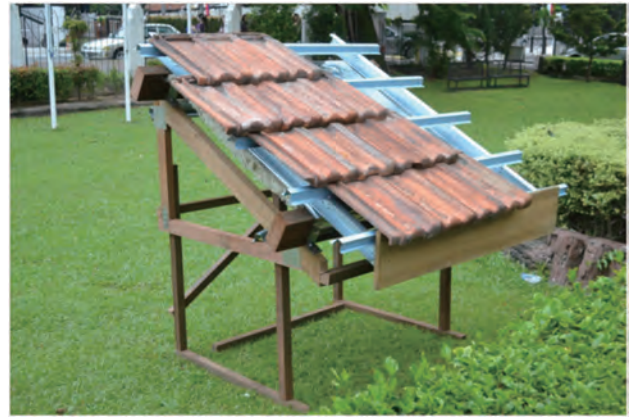
A roof mockup insulated with wire netting, rock wool and aluminum foil was set up at site for technical references
