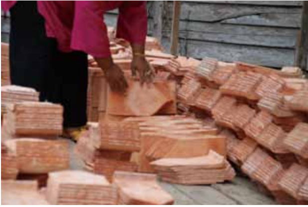
After removal from the kiln, each roof clay tile is inspected for possible overbaking or burning.
