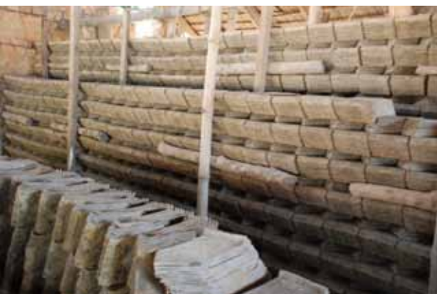
After sun drying, the good tiles are grouped together in packs of ten pieces and stacked horizontally in alternate order.
