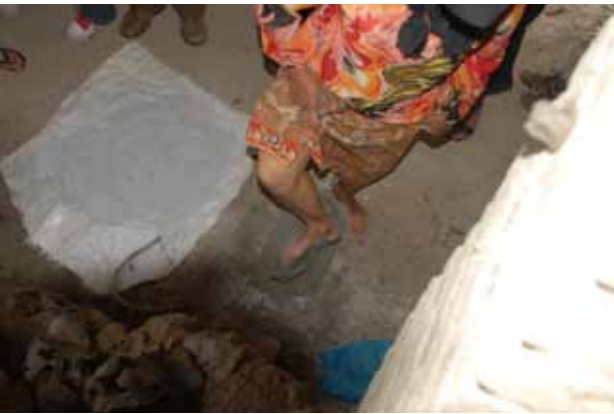
The roof clay tile maker places a slab of clay in the mould and presses the clay downwards a few times with her right foot to smooth out the clay.
