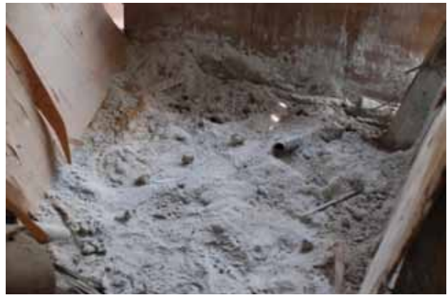
To prevent any clay from sticking onto the wooden mould, paddy husk ash is spread all over the wooden mould before the pressing process begins.
