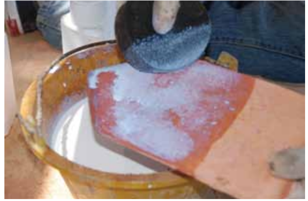
The roof clay tiles are treated with a water-resistant application before being transported to clients.
