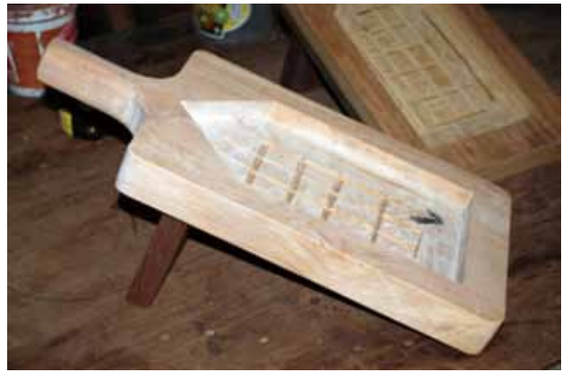
A wooden mould is used to shape the clay into its rhomboid-shaped signature design.
