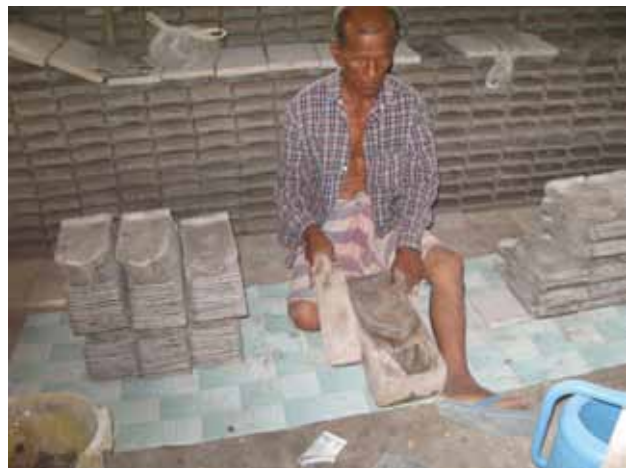
Once dried, the clay tiles are collected and inspected for possible defects.
