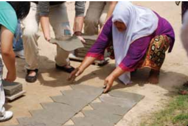
The grey clay sheets are laid down in rows on the ground under the hot sun of 32-35 degrees Celsius.
