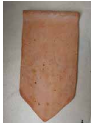
Bottom view of the Singgora roof clay tile with a small right angle of 28mm at the straight end.
