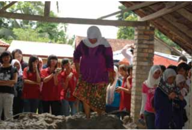
A roof clay maker uses her bare feet to wedge and knead the clay bundle.
