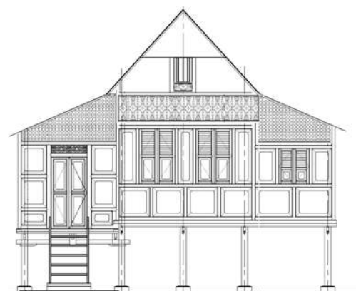
The right elevation of the Bugis house showing its external staircase leading to the entrance door, carved lattice panels, louvered casement windows of two sizes, double-layered gable end with a small window and a pitch roof.
