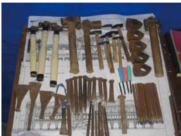
Tools used to remove the stubborn cement pointing, rake out incongruous mortar and carry out re-pointing in lime mortar
