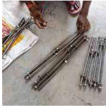
SS rods 500 mm long and 12 mm in diameter with nuts and bolts were used at 1 foot c/c distance, both vertically and horizontally, to hold the parts together
