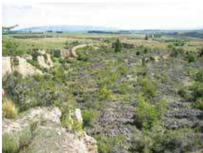
Figure 20. Sluice faces and extensive gold tailings resulting from the mining of an ancient river terrace using water under pressure sourced from reservoirs (Photo: Briden & Schmidt 2007).
