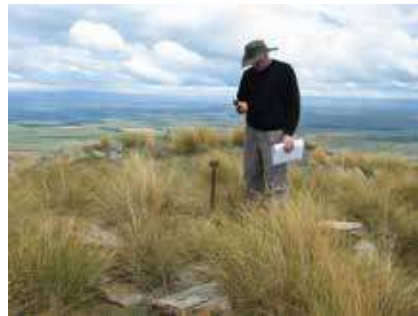
Figure 15. A 19 th century surveyor's trig marker (probably 1870s) high up in the mountain tussock. From these elevated points, land boundaries and mining claims were surveyed from and referenced (Photo: Briden & Schmidt 2007).
