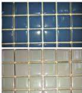
New blue glazed porcelain mosaics for the domes and grey glazed porcelain mosaics for the pyramid roofs that match the original mosaics. Each glazed porcelain mosaic measures 19 mm×19 mm with a slightly convex-edged design. The thickness of each glazed porcelain mosaic is 5 mm.
