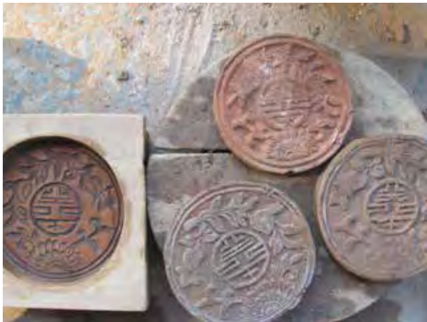
23. Wooden patterned molds to make roof tiles
