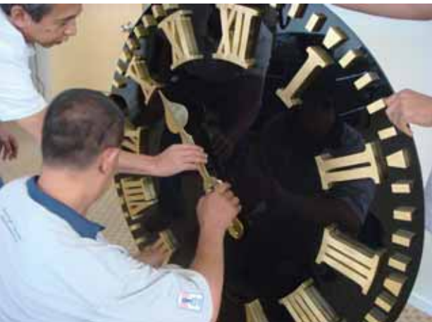
The new clock consists of aluminum minute markers, stainless steel Roman numerals; and stainless steel hour and minute hands which were all gilded with 23.5-carat gold leaf
