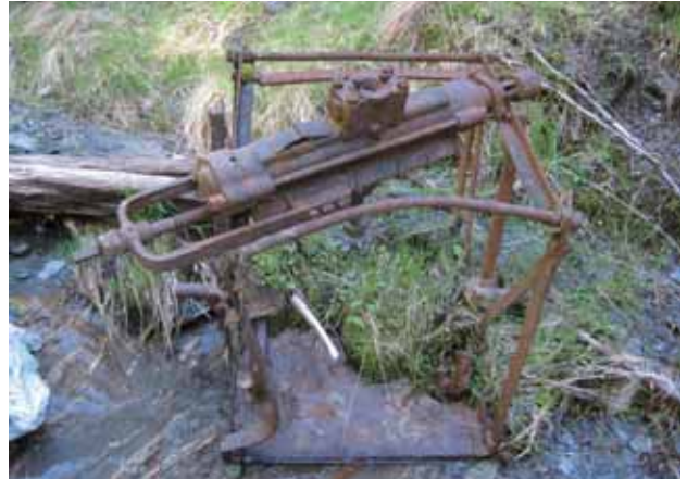
Figure 14. Author with Cornish rock drill still located next to the mining drive where it would have been used (Photos: Peter Petchey and Matthew Schmidt).
