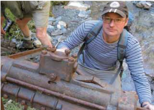
Figure 14. Author with Cornish rock drill still located next to the mining drive where it would have been used (Photos: Peter Petchey and Matthew Schmidt).
