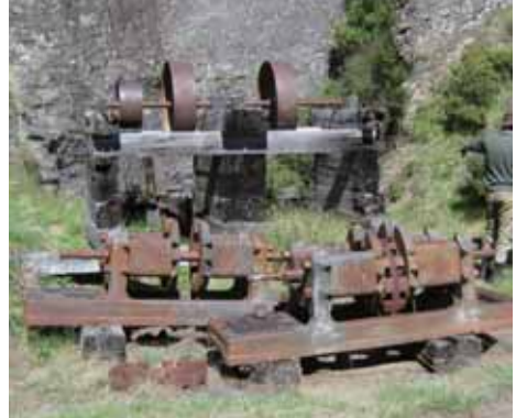
Figure 19. The Dynamos for the hydroelectric power scheme. Top: as drawn and published in the Appendices to the Journals of the House of Representatives in 1886; Bottom: as photographed by Matthew Schmidt in 2010.
