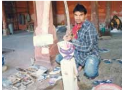
An inlay piece is cut using a bow string saw.
