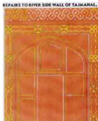
Documentation before restoration: Yellow is the existing and white is the missing inlay.
