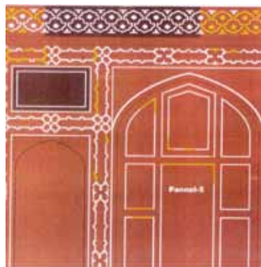
Post-restoration documentation (not of the same panel) : Chocolate is replaced base stone; white is the new inlay.
