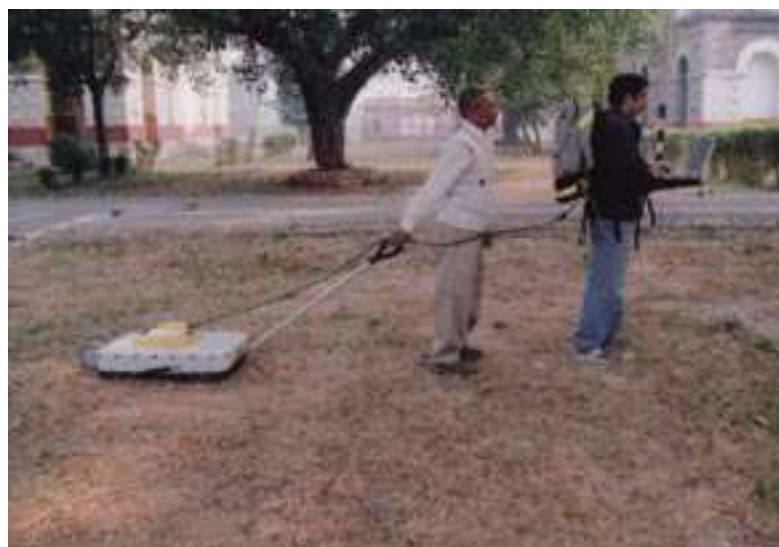
GPR survey was carried out before the excavation.
