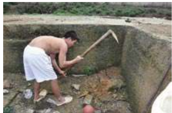
Picture 4: Exploitation of laterite at their own garden Duong Lam village - Hanoi
