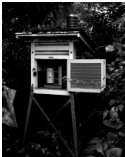
Fig.5 Metal and pigment test pieces in screen
