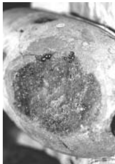
Fig.3. The Iron cannon ball excavated from sea and natural dried. Iron rust has increased rapidly.
