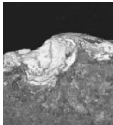
Fig.4. The bronze disease is formed with the chemical reaction of copper and the chloride ion.
