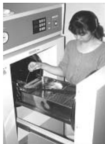
Fig.6.The High temperature and high pressure device. (chloride removal for iron objects.)
