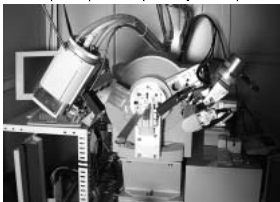
Fig.2. Non-destructive X-ray diffraction system
