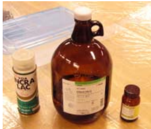
(From left to right:) BTA spray (commercial name: INCRA LAC), ethanol, and BTA.
