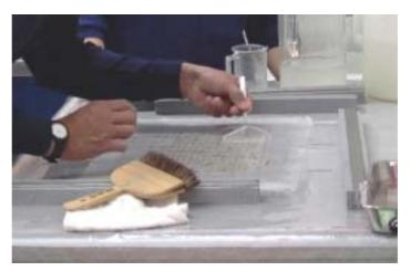
Remove all the temporary liners using tweezers.
