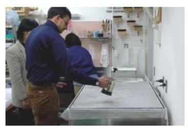
Seal the unused area of the suction table with plastic sheets for maximum suction effect.
