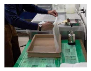
Place them on the designated area of the suction table from the far edge line towards the body with as little air intrusion as possible. Brush away the captured air with a dry flat brush.
