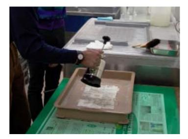
Wet them completely, smooth out creases with a flat brush, and pull the unwoven cloth out of the water together with the document on top.
