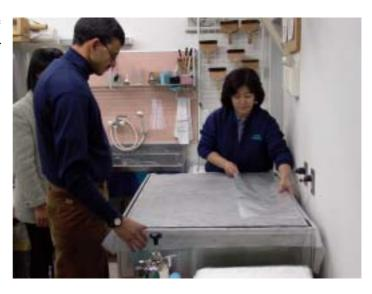
Place the dried document with temporary linings face down on the unwoven cloth. Float the two pieces together on a vat (square tray) filled with water, and spray water from above.
