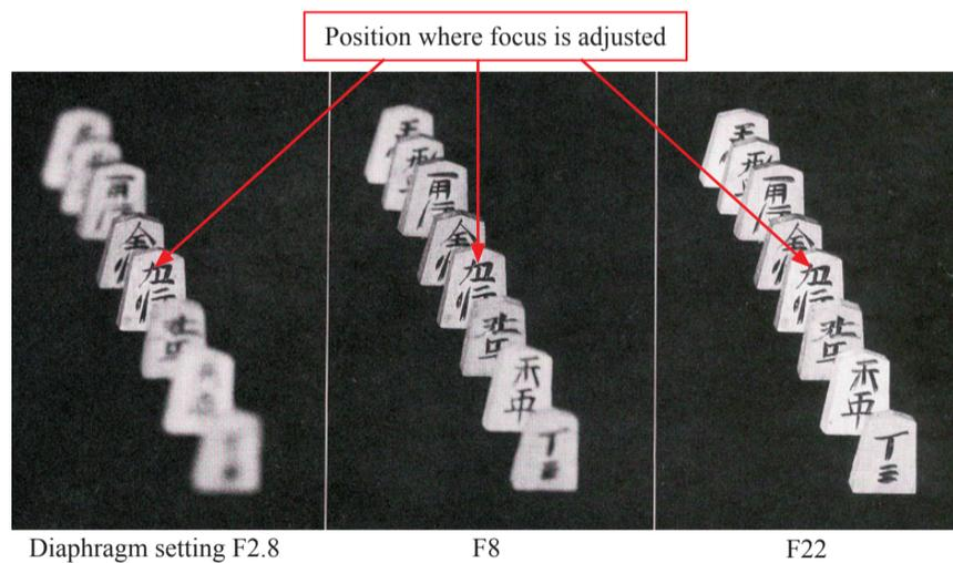
Fig. 7: Field depth and focus depth
