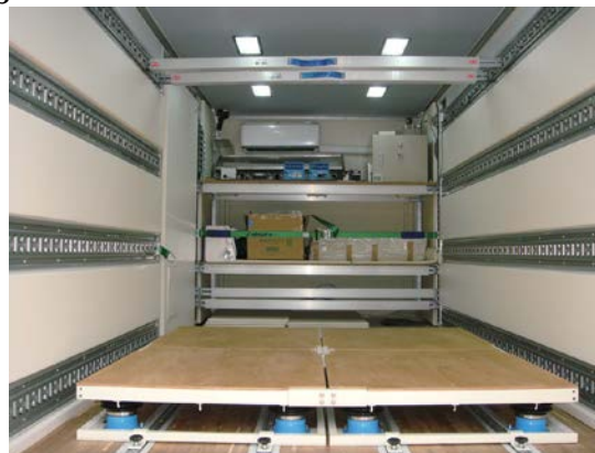
The vibration isolator and monitoring system ensure safe transportation. (Shvara II)
