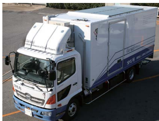
A 24-hour air conditioning system using solar panels is built in. (Shvara II)
