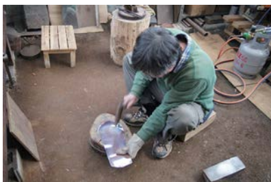
Beating out an iron plate of armour
