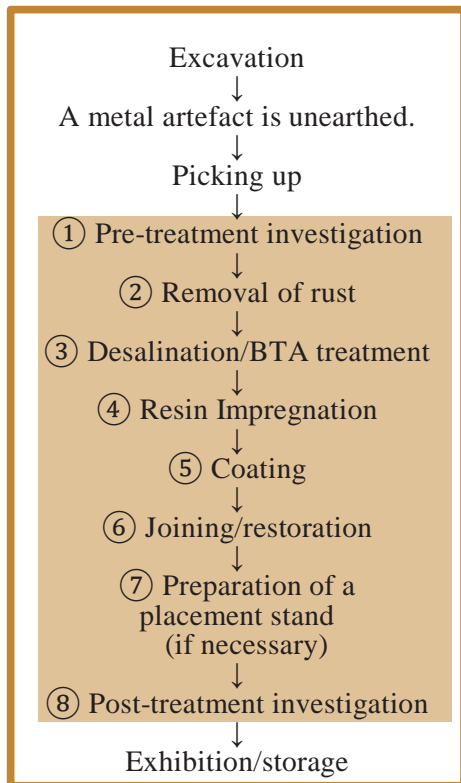
Conservation process for metal objects
