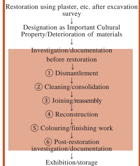
Conservation/restoration process for earthenware
