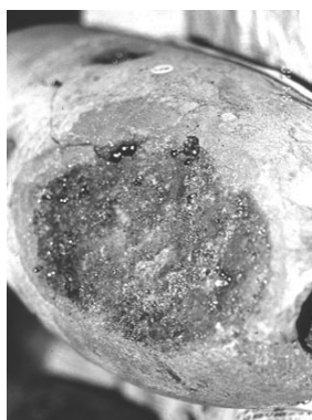
Fig.4: An Iron cannon ball excavated from the sea and dried naturally showing a rapid increase in iron rust.
