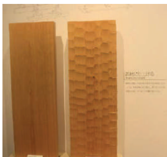
Fig.5 Difference of surface finishing using two different tools, as shown in Takeneka Carpentry Tools museum
