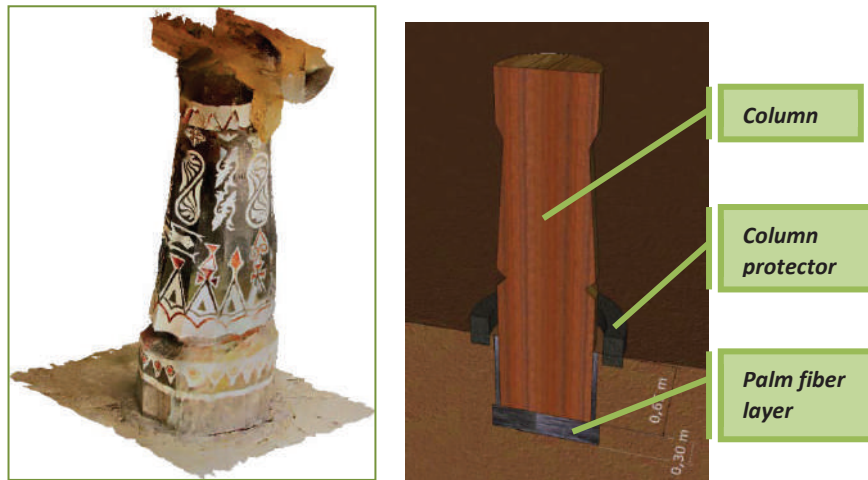
Fig.2 Partogu column 3D detail (left), and partogu column cross section detail (right)
