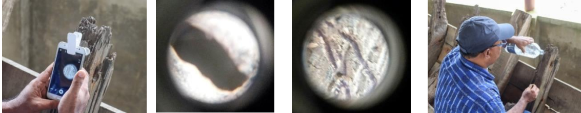
Figure 5: Examination the small wood cellular with a microscope and trying to remove the white spots with water.
