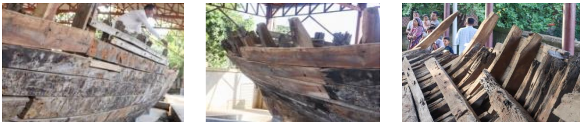
Figure 4: New wood additions in many places.
