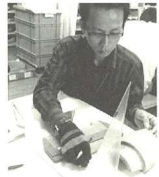
Measuring a flat tile with mako (left) and a round tile with a triangle ruler (right)
