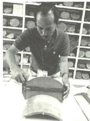
Measuring a flat tile with mako (left) and a round tile with a triangle ruler (right)
