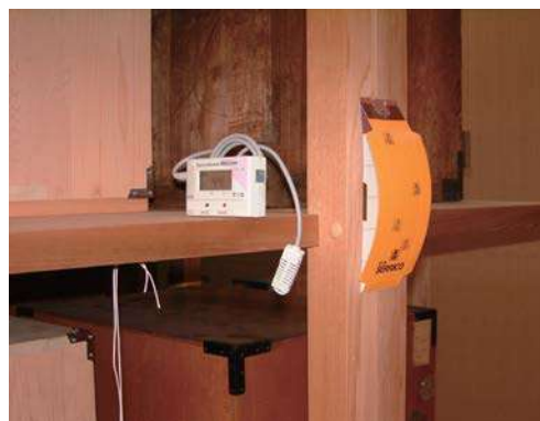
Temperature/humidity monitor (left) and pest detector (right)
