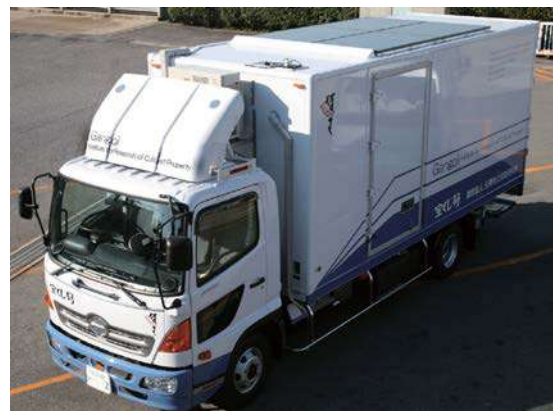
A 24-hour air conditioning system using solar panels is built in. (Shvara II)
