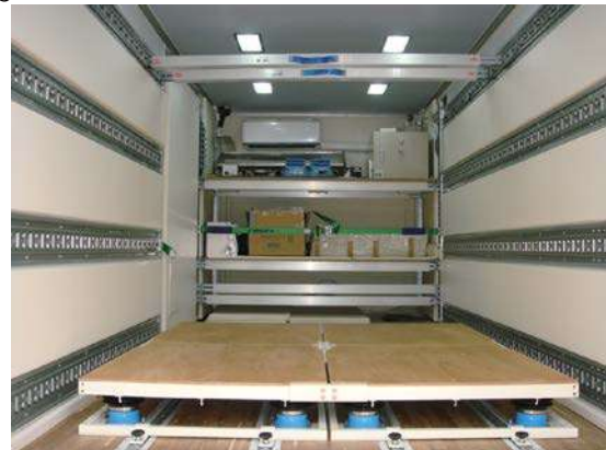
The vibration isolator and monitoring system ensure safe transportation. (Shvara II)
