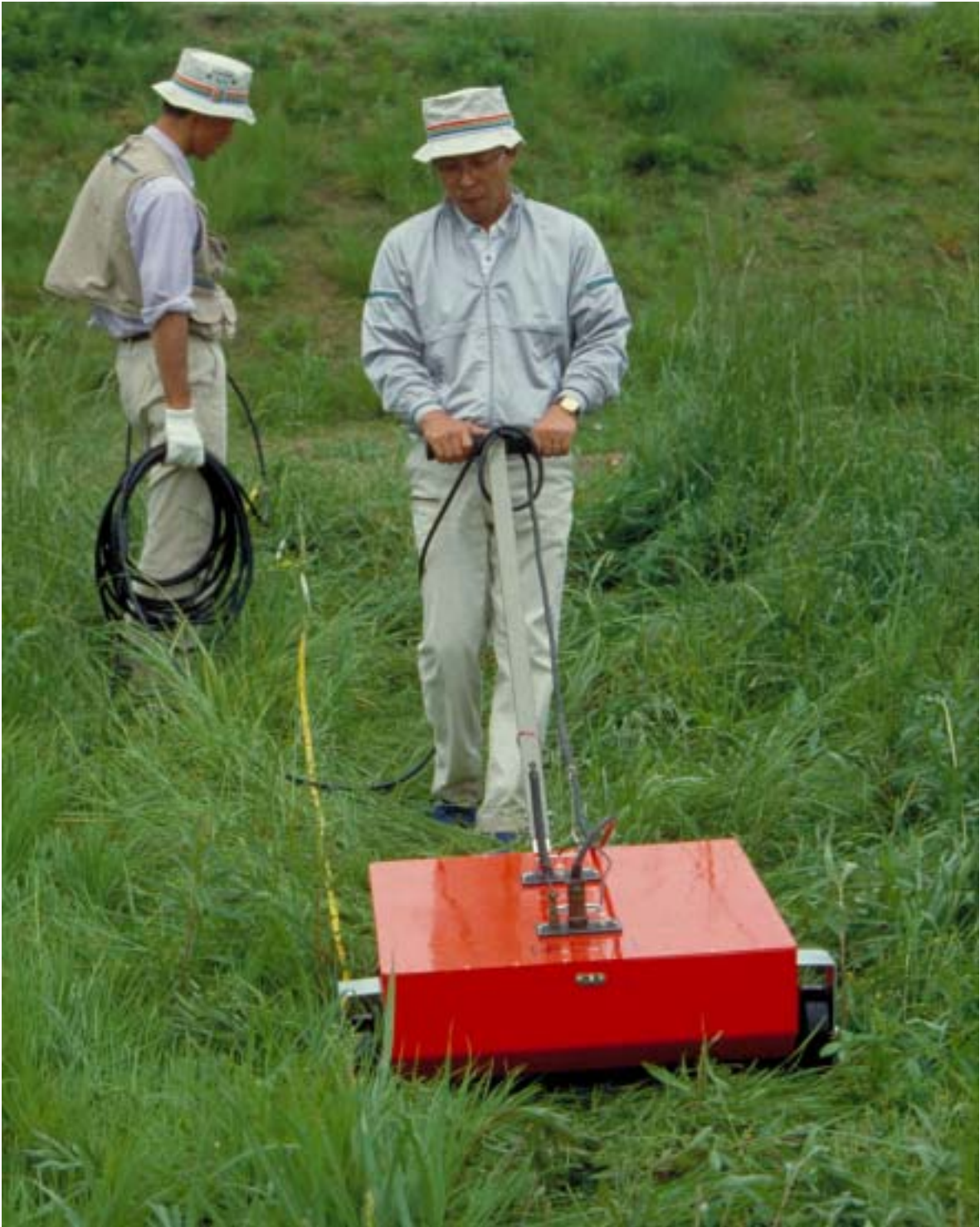
Ground Penetrating Radar Survey (GPR) 300MHz antenna
