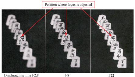
Fig. 7: Field depth and focus depth
