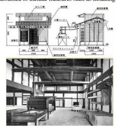
Fig.37 Fire Proof test for traditional wooden House (upper) and Hibukuro design in kitchen (lower)
