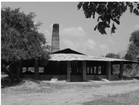
The brick kiln established to produce the ancient sized bricks)
