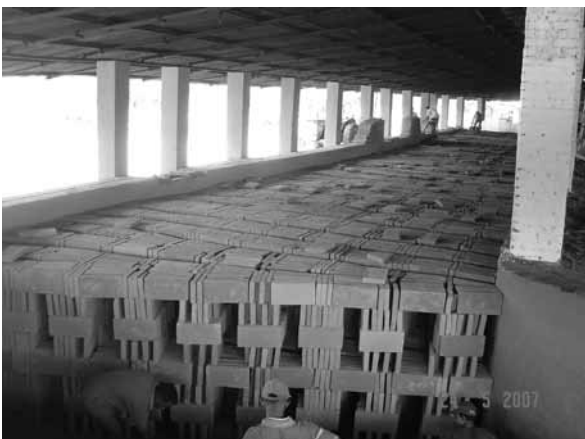
Stacked green bricks showing the gaps created for the movement of heat
