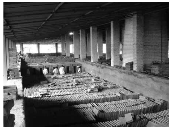
Stacking of green bricks for firing
