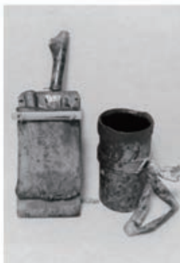
Fig.18. Tools for lacquer tapping (old stock of Kiyotaro Omori in Jobojimachi)
