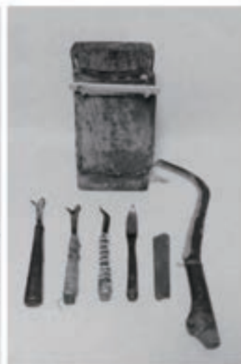
Fig.18. Tools for lacquer tapping (old stock of Kiyotaro Omori in Jobojimachi)
