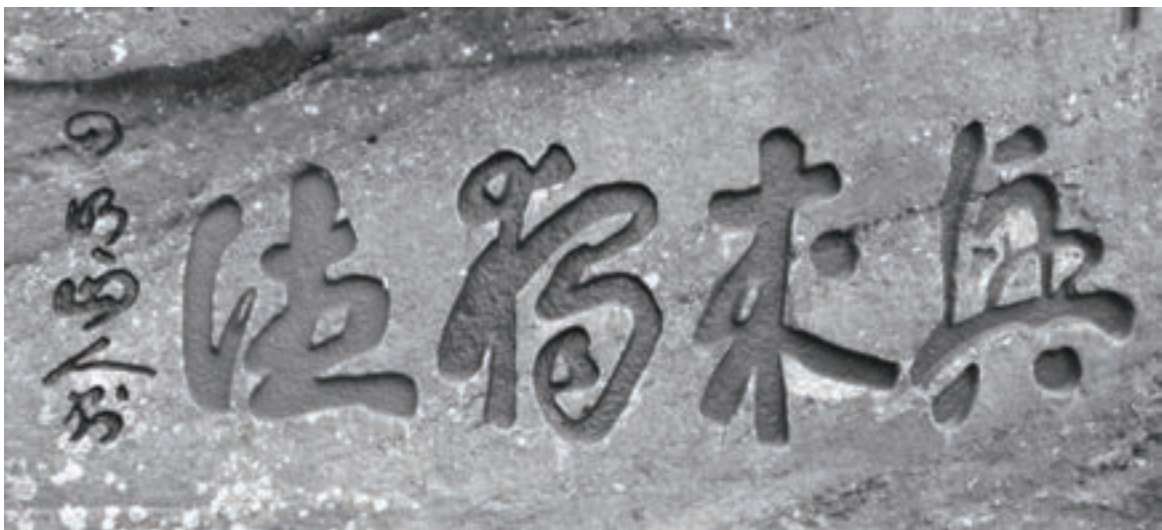
Figure 13. Inscription“兴来独往”: fading of different pigments one year later (the cinnabar in the left has turned dark purple)
