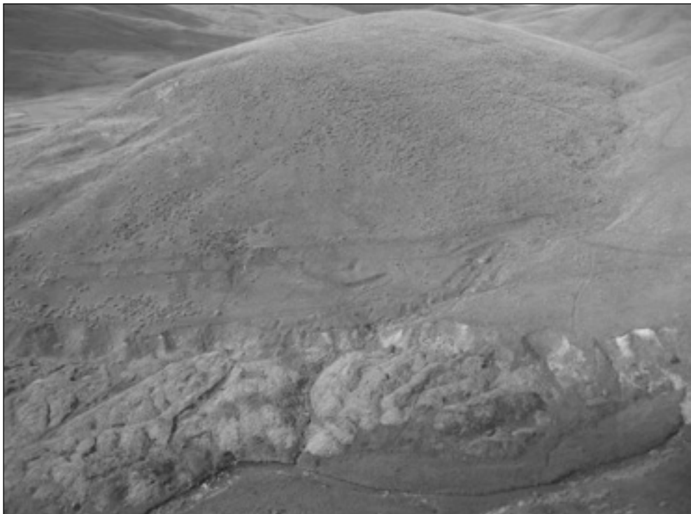
Figure 21. Aerial view of a 19 th century gold mining system in Otago. Water races, a reservoir, sluice faces and tailings can be seen. (photo: Shar Briden).
