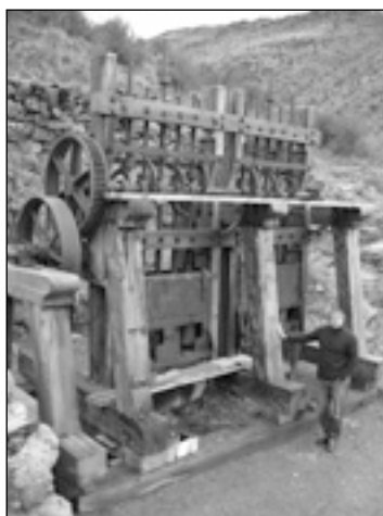
Figure 41. The Come-in-Time gold mining battery after restoration works ca. 11 months later. The replaced macrocarpa timbers will eventually weather and appear as the aged originals.
