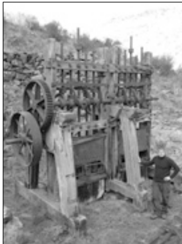
Figure 40. Come-in-Time gold mining battery, Bendigo, Central Otago. Before restoration works. (photo: Matthew Sole).
