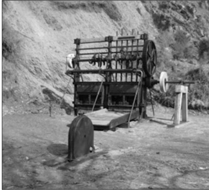
Figure 50. Metal gold mining battery after restoration works. (photo. Shar Briden)
