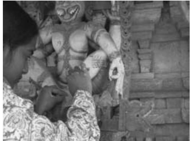
Fig. 14 Collecting samples of paint from a wooden sculpture to test the date and constituents
