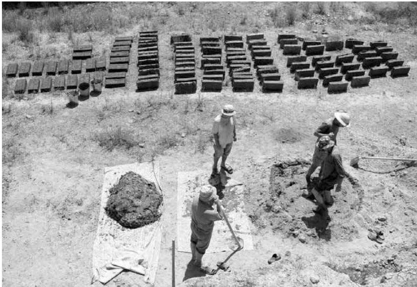
Figure 5. Process of making adobe bricks (Panjakent)
