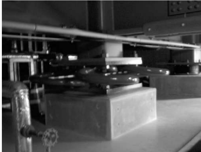
System to restore the building to its original position after an earthquake
