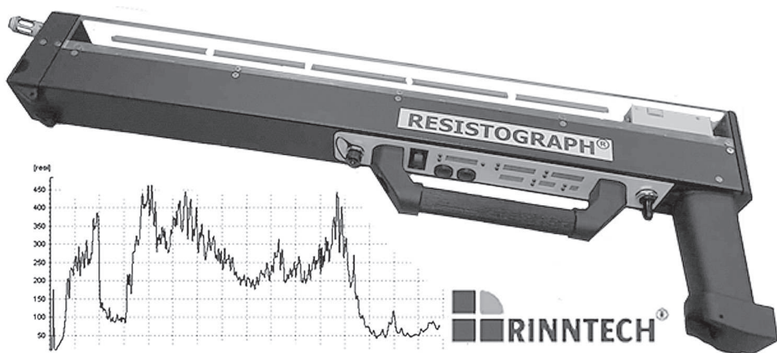
Figure 5. Resistograph measuring device and a reading from the Tango Monastery
