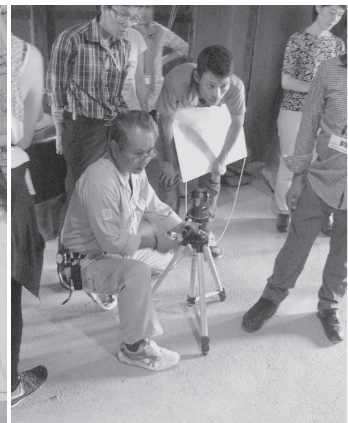
Mr Hamaguchi demonstrating measurement with a lazer level
