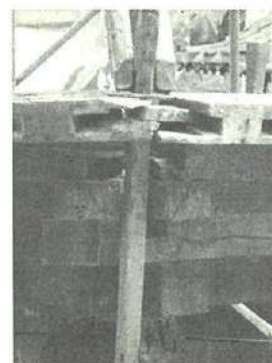
Pre-reconstruction with original material. Connection between takir in the corner was broken so the dudur cannot line its force.
