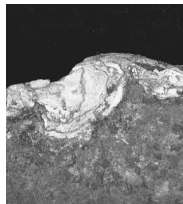
Fig.8. The bronze disease is formed with the chemical reaction of copper and the chloride ion.
