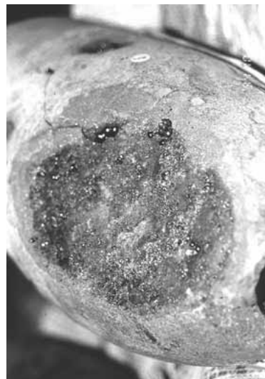
Fig.7. Iron rust has increased rapidly because the iron cannon ball recovered from sea was naturally dried.
