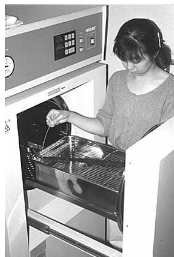
Fig.10. The High-temperature and high-pressure device. Chloride removal for iron.
