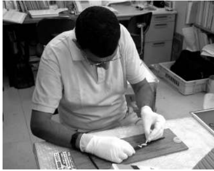
Filling of iron nail with epoxy resin
