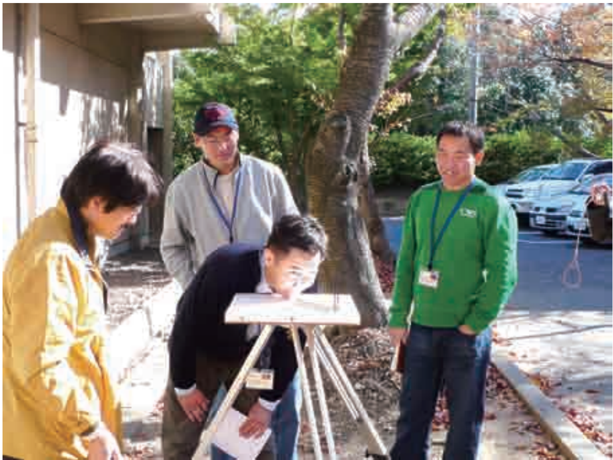
Practical training on plane-table surveying
