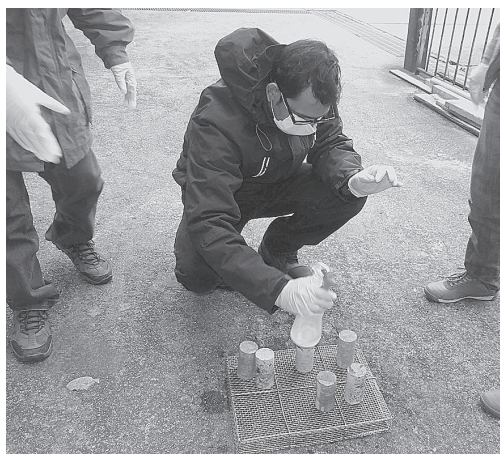
Applying water repellent agent
