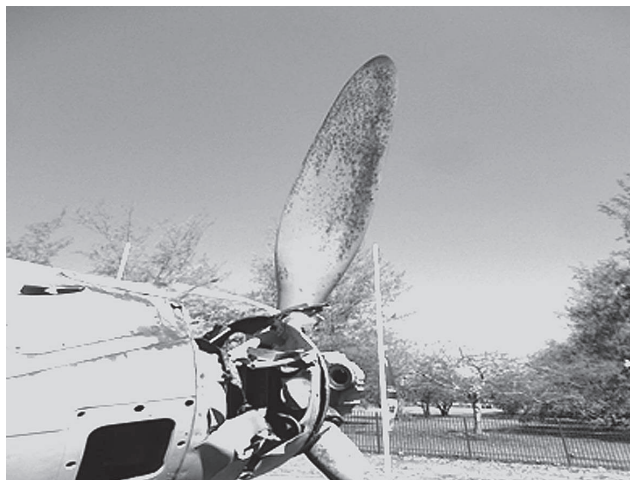
Figure 3. A WWII war plane showing signs of corrosion
