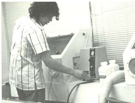
Cleaning of iron rust using the Airbrasive 6500
