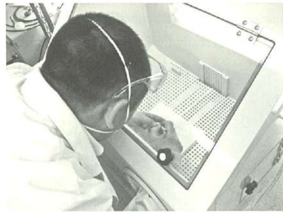
Cleaning of iron rust using the Airbrasive 6500
