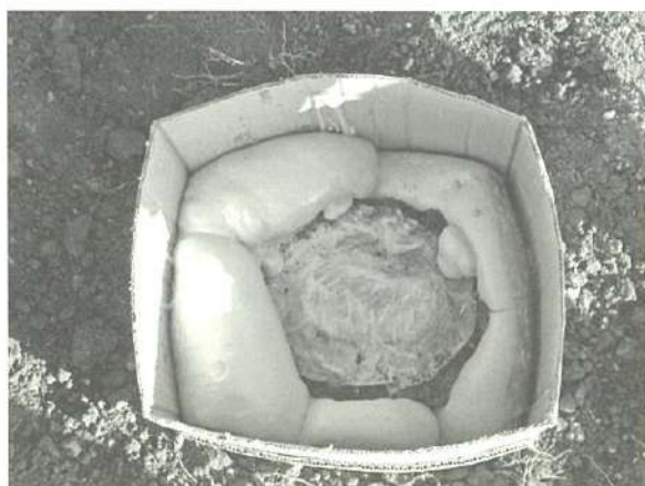
Urethane foams and solidifies to 10 times its original volume.
