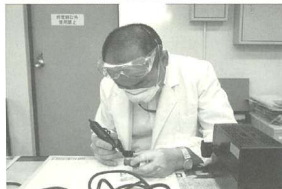
Practicing desalination treatment to bronze artefacts
