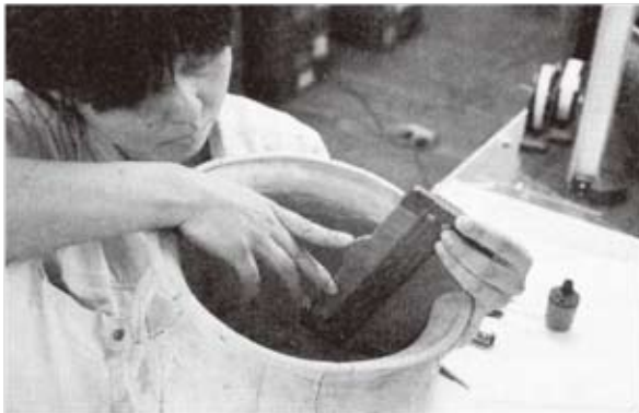
3. Gauge contours of earthenware with mako.
