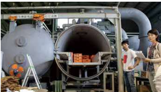
Observation of the conservation laboratory at NNRICP (Left:Optical microscope, Right:Vacuum freeze-drying chamber)
