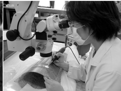
Removal of corrosion product by mechanical method
