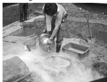
Taking out by using polyurethane foams and LN 2
