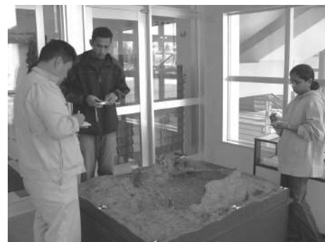
Assisting data taking for digital photogrammetry. Recoding the coordinates of targets set on the object
