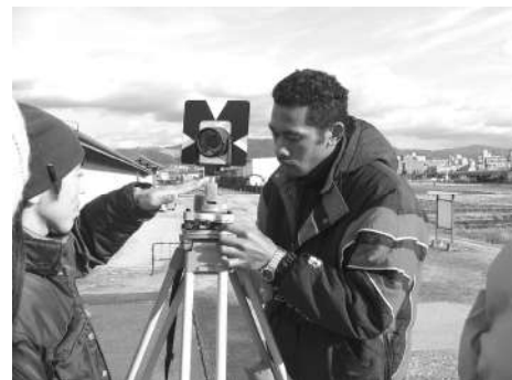
Setting the reflector for the Total Station
