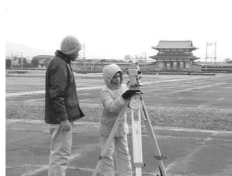
Fixing the Total Station on the benchmark, at Heijo Palace Site
