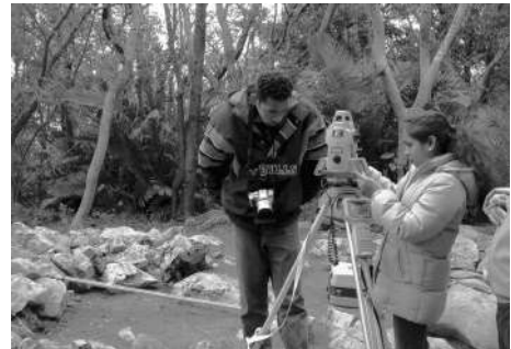
Topographical Survey by Total Station
