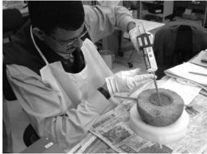
Joining pieces with adhesive resin
