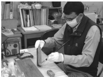
Cleaning the wood with brush: the first step for the treatment
