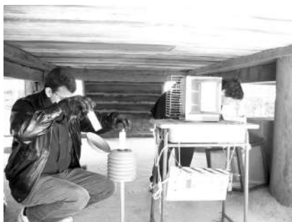
Replacement of TEA cylindrical filters
