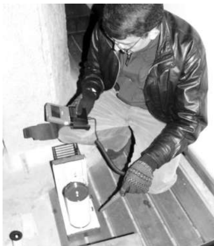
Checking the temperature to adjust the hydro-thermograph measurement machine
