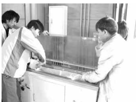
Iron objects were impregnated in resin solution.
