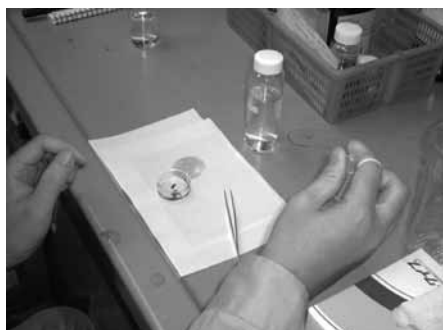
Making thin slices of a wood block for identification of tree species
