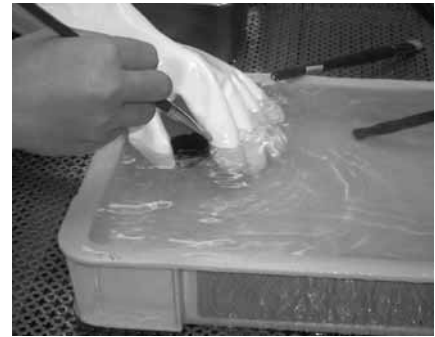
Washing off sugar on the surface in hot water
