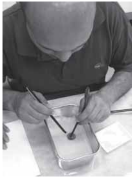
Mechanical cleaning of a bronze artefact with a graver(left) and a brush (right)
