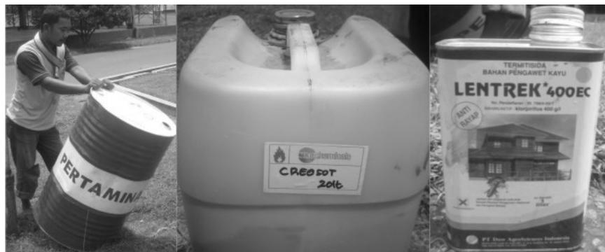
Chemicals used to prevent termites in Pendopo Ageng's restoration, as a mixture of kerosene, creosote, and Lentrek in the ratio 1:1:0.05
