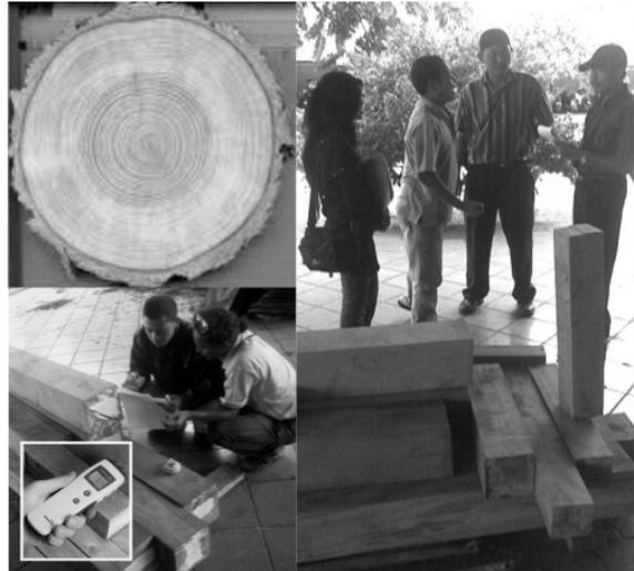
New teak wood for use to replace damaged components. The new teak wood must have the same quality as the original components and be at least 80 years old, with a moisture content of less than 14 percent. *Insert:* Protimeter, a tool for measuring the moisture content in wood.
