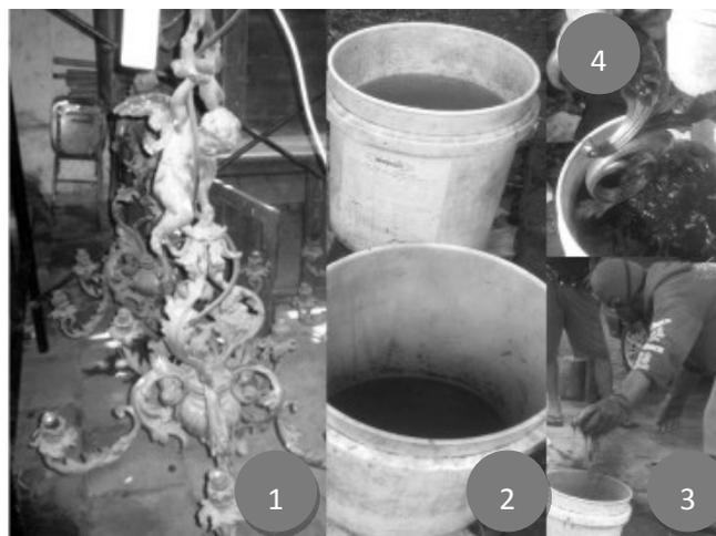
Conservation of a chandelier: (1) before conservation, (2) nitric acid (*top*) and sulfuric acid (*bottom*) used for conservation, (3) dipping parts in sulfuric acid, (4) dipping parts in nitric acid
