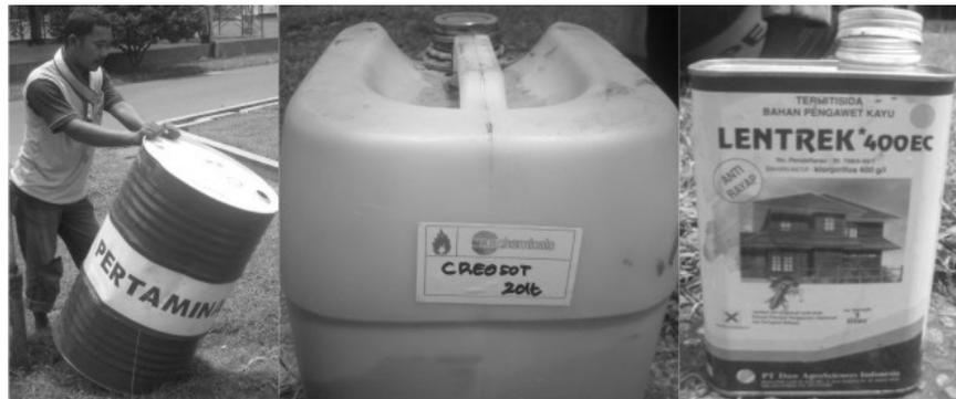
Chemicals used to prevent termites in Pendopo Ageng's restoration, as a mixture of kerosene, creosote, and Lentrek in the ratio 1:1:0.05
