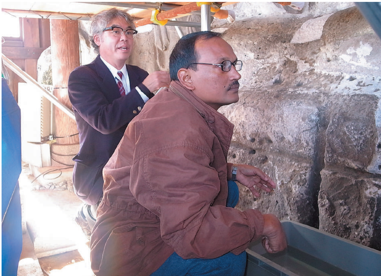
Observation of salt weathering at Motomachi Stone Buddhas (the white part shows salt crystallisation)
