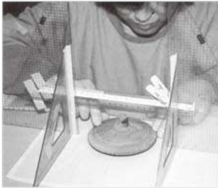
1. Set the earthenware on graph paper and measure the bore of it.
